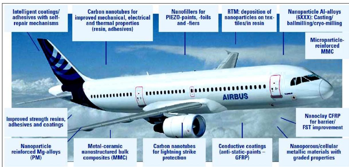
Figure 72 - Nano-materials applications in aircraft (Max Planck Institute 2009, 214)
